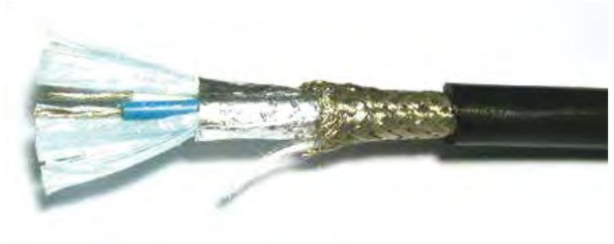
A suitable cable for this application is “BELDEN 82841” (nominal characteristic impedance 120 Ohms, nominal conductor DC resistance @ 20 °C 24 Ohms/1000 ft., max. recommend current 4 Amps per conductor @ 25 °C).
