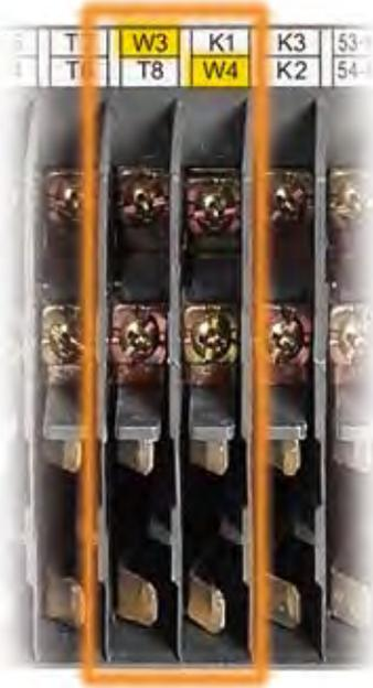
PR021/K module shall be connected to the internal bus of the trip unit, through the slots W3 and W4 of the terminal box (the figure shows the terminal box of a withdrawable circuit-breaker type Emax).
